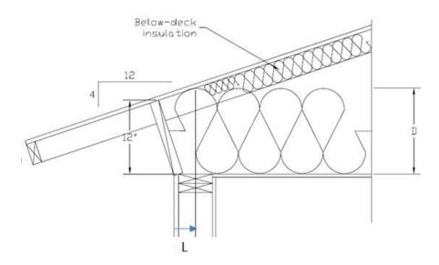
L and D determine where the top of the ceiling insulation meets the roof deck plane.
