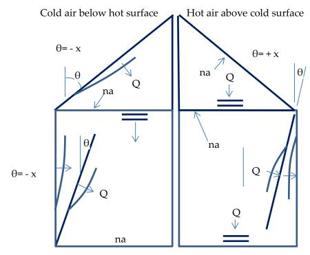
Figure 5: Heat Flow Up Situations
