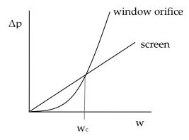
In Figure B-2, to the left of  $w_c$  the laminar-flow screen pressure drop is higher, and to the right the orifice pressure drop dominates.
