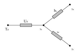
The temperatures of the duct zone are assumed to be constant; the duct surface temperature is not. The duct surface temperature can be removed from the analysis by using a Y- $\Delta$  transform. Figure A-2 shows the result of this transformation with direct connections between the duct air temperature, the duct zone radiant and air temperatures through combined coefficients defined in Equation A- 1.
