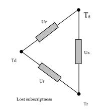
Figure A-2: Heat Transfer through a Duct Wall with Surface Temperature Removed
