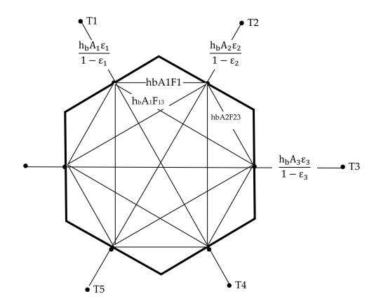
Figure C-2: View-Factor Method's Network for Grey Surfaces
