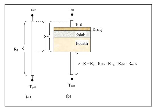
Figure 20: Addition of Film, Rug, Slab, and Earth
