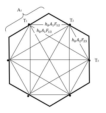
Figure C-1: View-Factor Method's Radiant Network for Black-Body Surfaces
