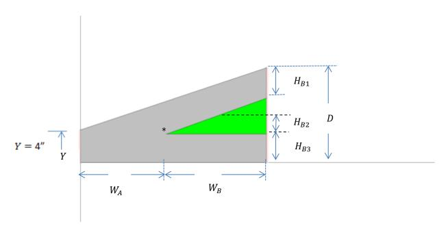
Figure 30: Standard-Heel Simplified Geometry for Framing Path
